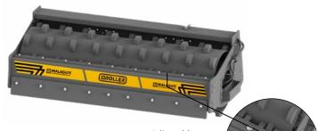
Adjustable scarifier drum cleaning High-performance vibrating roller with a drum with **padfoot drum**, particularly suitable for compacting cohesive soils, such as clay and loam, during construction work. It is also usable for maintaining unpaved roads
